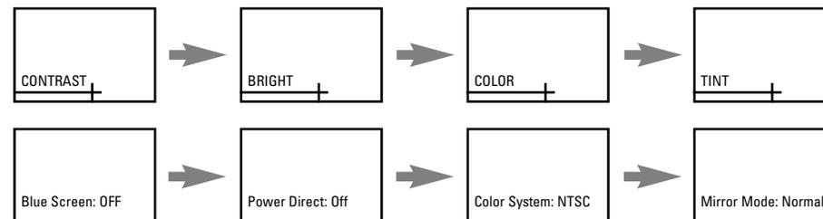
Adjust each function, CONTRAST, BRIGHTNESS, COLOR, TINT, ON/OFF, NTSC/PAL, NORMAL, MODE SELECTOR with VOL (+ -) button.
