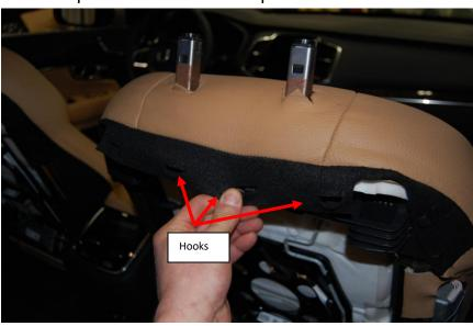
• By flipping the material up towards the headrest you will be able to locate the plastic release clips for the headrest.
